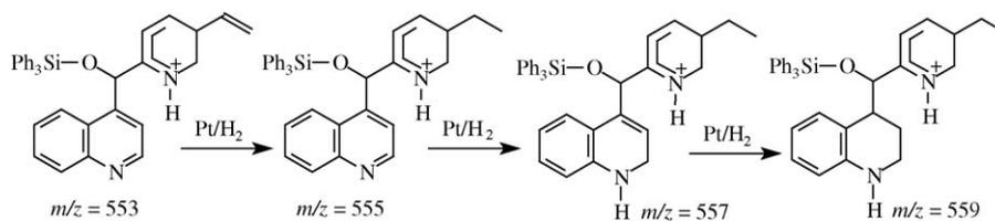
Fig. 6. Formed hydrogenated derivatives in the hydrogenation of Ph<sub>3</sub>Si-O-CD on Pt-alumina catalyst (standard conditions).
