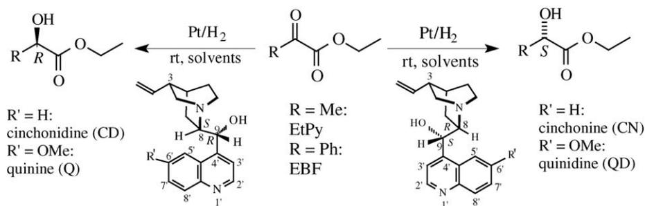
Fig. 1. The Orito-reaction ( $R = Me$  (ethyl pyruvate = EtPy,  $R = Ph$  (ethyl benzoylformate = EBF)).
