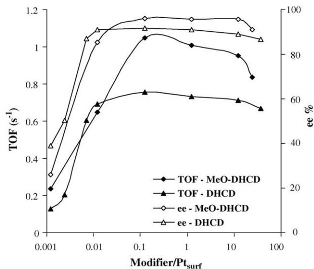
Fig. 4. Initial rate and enantioselectivity as function of Modifier/Pt<sub>surface</sub> for hydrogenation of EtPy (for conditions and abbreviations, see Fig. 3).
