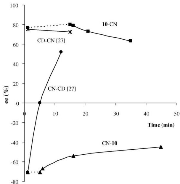
Fig. 7. Enantioselective hydrogenation of EtPy: effect of modifier mixtures (standard conditions, 273 K, 3 ml THF, [CN] and [**10**] (containing 0.2% CD): 0.1 and 0.1 mmol/l, first abbreviation-modifier used first, second abbreviation-modifier added afterwards).
