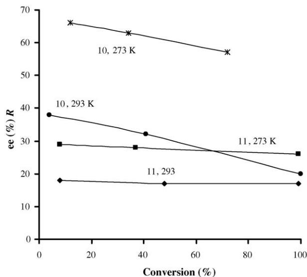
Fig. 5. Enantioselective hydrogenation of EtPy on Pt-alumina catalyst modified by **10** (containing ~0.7% CD) and **11** (containing 0.2–0.3% DHCD) cinchona derivatives: effect of conversion and temperature on ee (standard conditions, solvent THF, [**10**, **11**]: 0.1 mmol/l).
