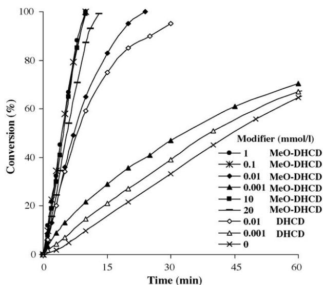
Fig. 3. Enantioselective hydrogenation of EtPy on MeO-DHCD (**2**) modified platinum (25 mg E 4759, 1 bar H<sub>2</sub>, 2 ml AcOH, 0.1 ml EtPy, 296 K).
